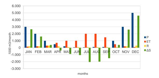
Figure 2. Example of a catchment water balance with monthly resolution (same input data used in figure 1)
