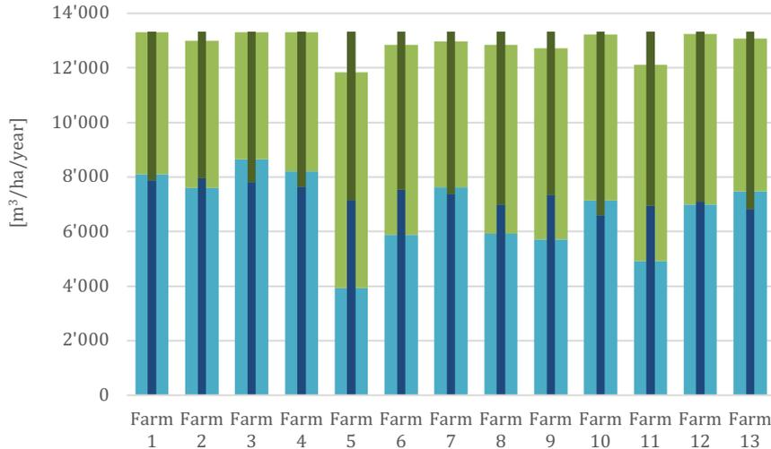
**Figure 6.** Annual blue and green water use and crop water requirement in the 13 banana plantations. Note: thin bars represent the irrigation scheduling scenario, and thick bars the actual water consumption.
